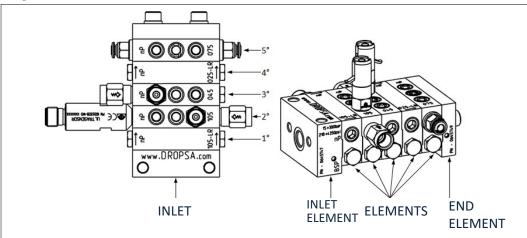
Note: to determine the left and right outlets, be noted that the assembly is seen vertically and metering elements are numbered sequentially starting from the bottom (inlet).
