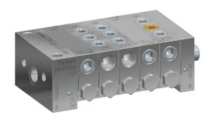
**nP** is a distributor that allows the feed flow rate be regulated in order to dispense very precise amounts to diverse outlets by means of the progressive movement of coupled pistons with micrometre-sized gears on the inside of the sliding hole.
