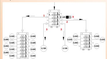
The **nP105** metering element (1) pilots a block of 6 metering 0,025 nP delivering elements and one 0,045 nPr.
