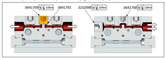
It is also possible to combine the flow rates of a metering element with the next metering element in the assembly by selecting an appropriate bridge metering element.
