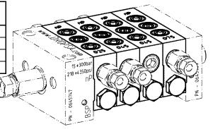
It's possible to combine the outlets into a single outlet by element replacing the yellow adaptor (Part number 0641709+0641791) with the white one as shown in the drawing below.
