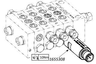
B) Visual monitoring pin with colour strip. This must be ordered with the divider element.
