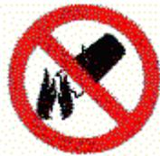
In case of fire, DO NOT use WATER, but the specific extinguishers for live equipment
