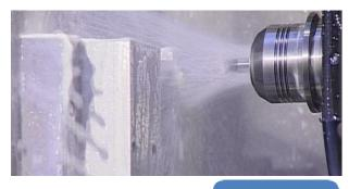
With *External* Lubrication: oil is transported via a nozzle to the cutting surface.
