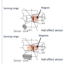
Normally, the magnetic field is balanced around the hall sensor. With the spool in the sensing range, the flux density is modified allowing the Hall Effect sensor to detect the presence of the spool. The use of a magnetic flex variation allows an extended sensing zone which avoids problems on systems with low flow rates and backpressure where the spool can often stop or bounce on the sensing surface.
